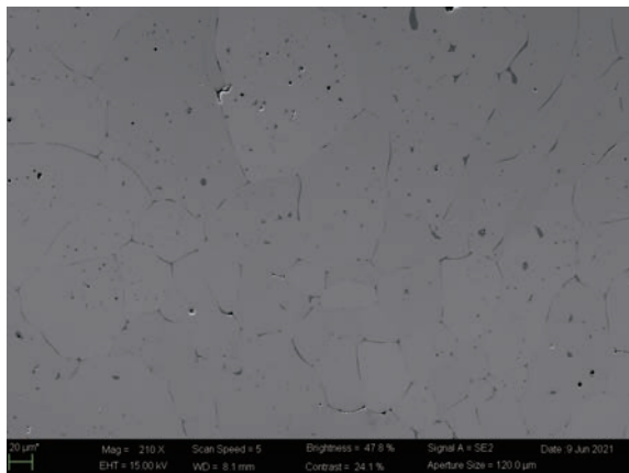
Fig. 1 SEM of Ni-Nb-Fe precursors prepared by arc melting
